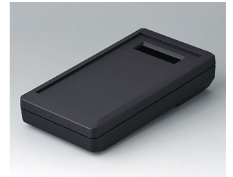
A9073319 DATEC-MOBIL-BOX S, Ausf. III ABS (UL 94 HB) schwarz RAL 9005 152x83x33,5mm IP 65 opt.
