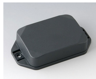
B1824228 MINI-DATA-BOX EF50, high, with flanges ASA+PC (UL 94 V-0) anthracite grey RAL 7016 70x50x20mm IP 65 opt., IP 40
