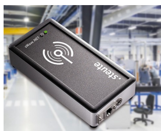
Wireless network access point
