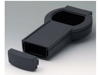
A9079209 DATEC-CONTROL L, Vers. II ABS (UL 94 HB) black RAL 9005 266x144x60mm IP 54 opt.
