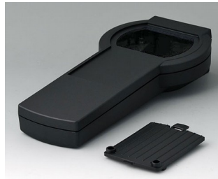
A9076209 DATEC-CONTROL XS, Vers. II ABS (UL 94 HB) black RAL 9005 200x94x40mm IP 65 opt.
