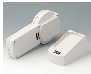
A9077157 SET: DATEC-CONTROL S, Vers. I, station.. ABS (UL 94 HB) off-white RAL 9002 228x117mm IP 65 opt.
