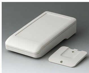
A9006207 DATEC-COMPACT M ASA+PC (UL 94 V-0) off-white RAL 9002 172x92x39mm IP 65
