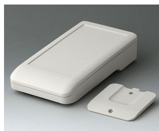
A9006217 DATEC-COMPACT M ASA+PC (UL 94 V-0) off-white RAL 9002 172x92x39mm IP 41
