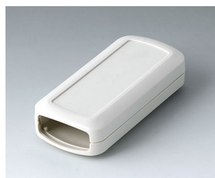
B2823107 CONNECT S ASA+PC (UL 94 V-0) off-white RAL 9002 90x42x22mm
