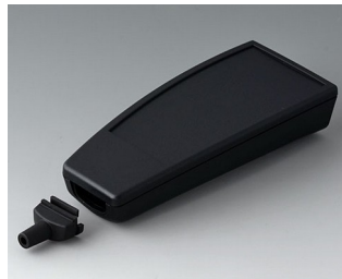
A9067329 SMART-CASE L, Vers. III ABS (UL 94 HB) black RAL 9005 140x62,7x30,5mm IP 65 opt., IP 40
