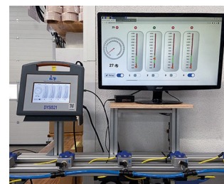
Monitoring system for cleaning nozzles
