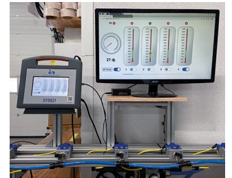
Monitoring system for cleaning nozzles
