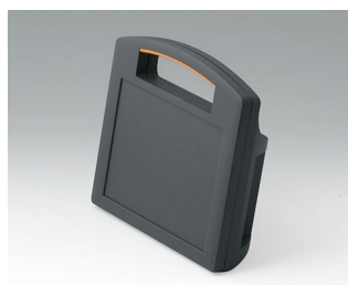
B4208208 CARRYTEC S ASA+PC (UL 94 V-0) lava 222x205x80mm IP 54 opt.
