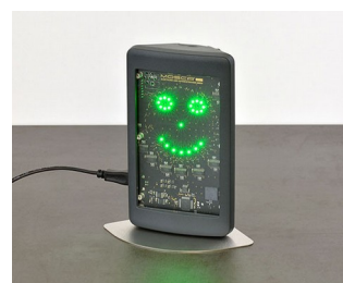
Room air measuring device
