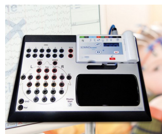
Stationary system for long-term EEG recordings
