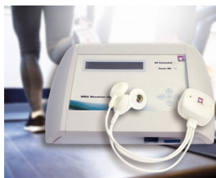
WBA receiver unit for measuring biosignals
