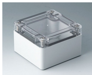
C7008014 IN-BOX ABS/PC (UL 94 HB) light grey RAL 7035 84x82x55mm IP 66, IP 67, IK 07
