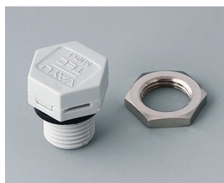
C2310917 Pressure equalisation element M10x1 PA 6 (UL 94 HB) light grey RAL 7035 IP 56
