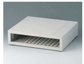
B2210017 MEDITEC D 220, without handle bar ABS (UL 94 HB) off-white RAL 9002 290x260x74mm IP 40
