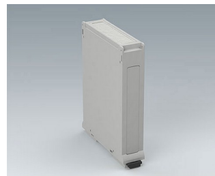
B6522101 RAILTEC BP, M22, with closed side panels PC (UL 94 V-0) light grey RAL 7035 95x23x113mm
