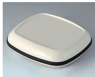
B1608217 BODY-CASE XL, with recess ASA (UL 94 HB) traffic white RAL 9016 62x56x17mm IP 65
