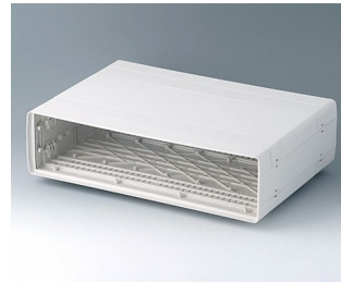
A0226070 EURO CASE 63 TE, without handle ABS (UL 94 HB) off-white RAL 9002 367x250x98,5mm
