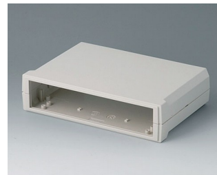
B3020117 MOTEC M, flat/flat ABS (UL 94 HB) off-white RAL 9002 205x140x50mm IP 40
