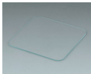
C6502013 Glass panel S84 Glass clear 78,75x78,75x1,6mm
