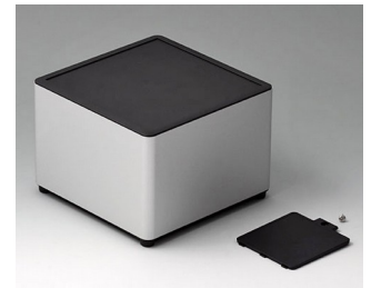
ES149059 SYNERGY S140 Aluminium AIMgSi 0,5 matt eloxiert 140x140x100mm IP 40
