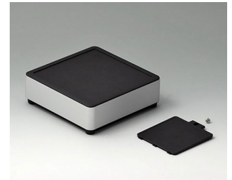
ES103059 SYNERGY S100 Aluminium AIMgSi 0,5 matt eloxiert 100x100x40mm IP 40
