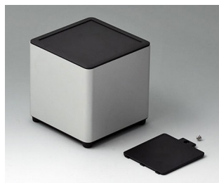
ES109059 SYNERGY S100 Aluminium AIMgSi 0,5 matt eloxiert 100x100x100mm IP 40
