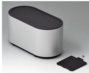
EO209059 SYNERGY O200 Aluminium AlMgSi 0,5 matt eloxiert 200x100x100mm IP 40
