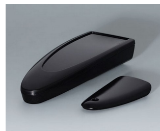
B2803016 STYLE-CASE M PMMA (IR) (UL 94 HB) schwarz RAL 9005 147x56x27mm IP 65 opt., IP 40
