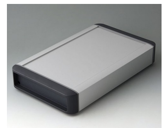
B3407032 SMART-TERMINAL 240 Aluminium AlMgSi 0,5 matt eloxiert 282x170x50mm IP 54
