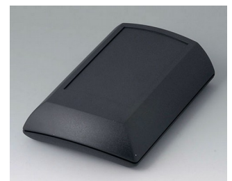
B7010209 ERGO-CASE M, flach ABS (UL 94 HB) schwarz RAL 9005 150x100x40mm IP 54 opt.
