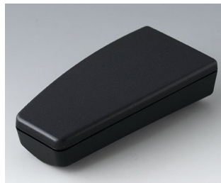
A9066209 SMART-CASE M, Ausf. I PMMA (IR) (UL 94 HB) schwarz RAL 9005 96x47x24mm IP 40
