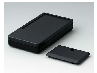
A9072119 DATEC-POCKET-BOX L ABS (UL 94 HB) schwarz RAL 9005 120x65x22mm IP 54
