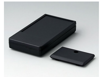
A9071219 DATEC-POCKET-BOX M PMMA (IR) (UL 94 HB) schwarz RAL 9005 105x58x18,5mm IP 54
