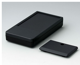
A9072109 DATEC-POCKET-BOX L ABS (UL 94 HB) schwarz RAL 9005 120x65x22mm IP 41
