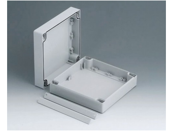
C2016162 ROBUST-BOX 160 BREIT, Ausf. II PC (UL 94 HB) lichtgrau RAL 7035 160x160x60mm IP 66
