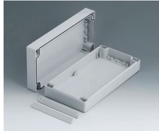
C2012242 ROBUST-BOX 120 BREIT, Ausf. II PC (UL 94 HB) lichtgrau RAL 7035 240x120x60mm IP 66
