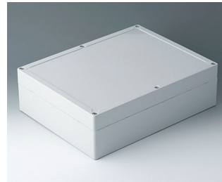
C7030101 IN-BOX ABS (UL 94 HB) lichtgrau RAL 7035 302x232x90mm IP 66, IP 67, IK 07
