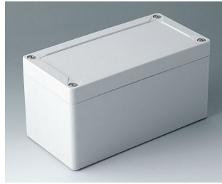
C7016021 IN-BOX ABS (UL 94 HB) lichtgrau RAL 7035 162x82x85mm IP 66, IP 67, IK 07
