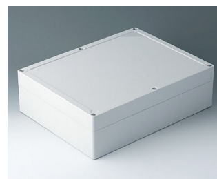
C7030102 IN-BOX PC lichtgrau RAL 7035 302x232x90mm IP 66, IP 67, IK 08
