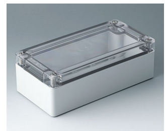
C7016014 IN-BOX ABS/PC (UL 94 HB) lichtgrau RAL 7035 162x82x55mm IP 66, IP 67, IK 07
