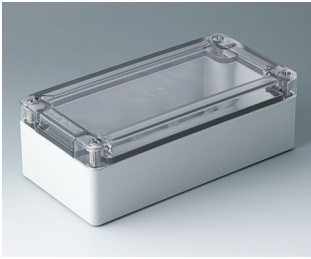
C7016015 IN-BOX PC lichtgrau RAL 7035 162x82x55mm IP 66, IP 67, IK 08
