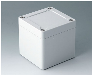
C7008021 IN-BOX ABS (UL 94 HB) lichtgrau RAL 7035 84x82x85mm IP 66, IP 67, IK 07
