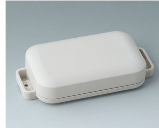
C3206107 EASYTEC 100 ASA+PC (UL 94 V-0) grauweiß RAL 9002 121x62x26mm IP 65 opt., IP 40
