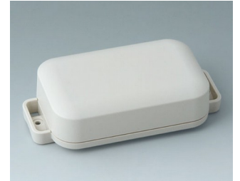
C3206207 EASYTEC 100 ASA+PC (UL 94 V-0) grauweiß RAL 9002 121x62x31mm IP 65 opt., IP 40
