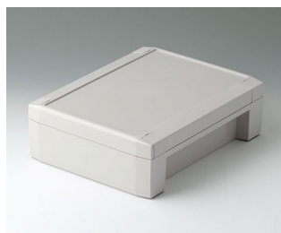
C8017222 SOLID-BOX 175 PC+ABS (UL 94 V-0) lichtgrau RAL 7035 225x175x70mm IP 66, IP 67, IK 08
