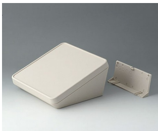
B4418207 PROTEC 180, Ausf. II ASA+PC (UL 94 V-0) grauweiß RAL 9002 180x180x92mm IP 65 opt.
