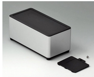
EE166059 SYNERGY E160 Aluminium AIMgSi 0.5 matt anodised 160x80x70mm IP 40
