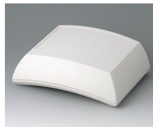
B7025207 ERGO-CASE L, high ABS (UL 94 HB) off-white RAL 9002 150x200x69mm IP 54 opt.
