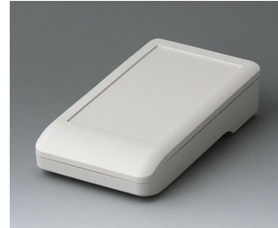
A9005117 DATEC-COMPACT S ASA+PC (UL 94 V-0) off-white RAL 9002 136x74x32mm IP 41
