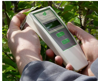
Chlorophyll fluorimeter for plant screening
