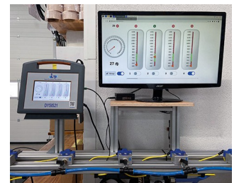
Monitoring system for cleaning nozzles
