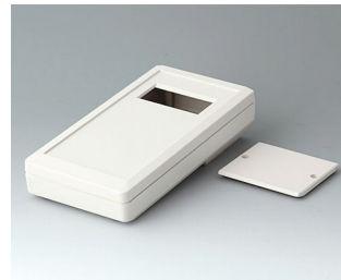
A9074407 DATEC-MOBIL-BOX M, Vers. IV ABS (UL 94 HB) off-white RAL 9002 195x101x44mm IP 65 opt.
