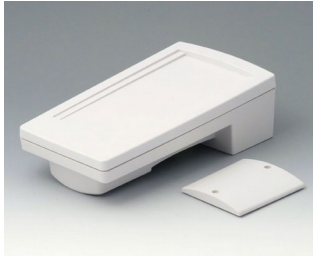
A9046107 HAND-TERMINAL M, Vers. I PC+ABS (UL 94 V-0) off-white RAL 9002 220x120x65mm IP 65 opt.
