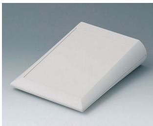
A0615007 COMTEC 150 F, Vers. I ABS (UL 94 HB) off-white RAL 9002 150x200x51.5mm IP 40
