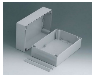
C2416241 ROBUST-BOX WIDTH 160, Vers. I ABS (UL 94 HB) light grey RAL 7035 240x160x120mm IP 66
