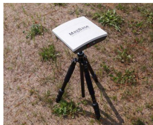
Measuring station for stationary field measurements
