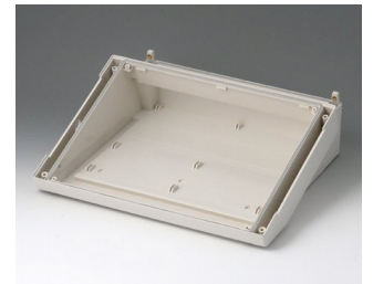
B4030317 DATEC-TERMINAL L, Vers. III ABS (UL 94 HB) off-white RAL 9002 302x272x101mm IP 54 opt.
