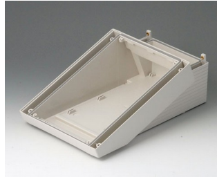
B4016117 DATEC-TERMINAL M, Vers. I ABS (UL 94 HB) off-white RAL 9002 168x272x101mm IP 54 opt.
