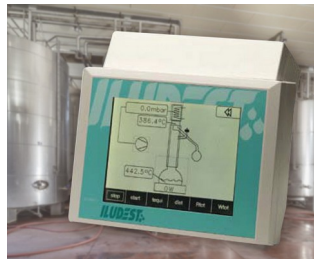
Device for monitoring and controlling distillation units
