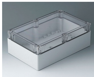
C7025084 IN-BOX ABS/PC (UL 94 HB) light grey RAL 7035 252x162x90mm IP 66, IP 67, IK 07
