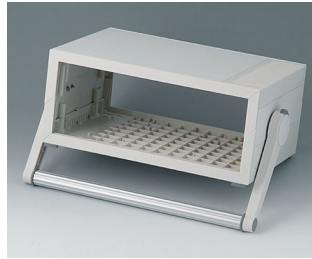
B2211307 MEDITEC D 160, with handle bar ABS (UL 94 HB) off-white RAL 9002 290x200x124mm IP 40
