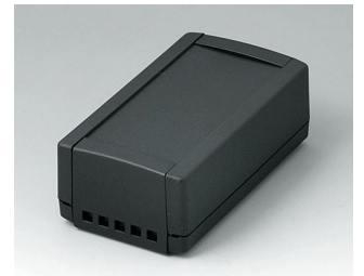
B1050469 TOPTEC 123 H, Vers. II ABS (UL 94 HB) black RAL 9005 123x68x45mm IP 40
