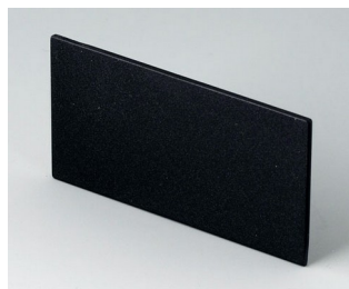
B6132222 Rear panel PPO (UL 94 V-0) black RAL 9005 73.6x39.75x1.7mm
