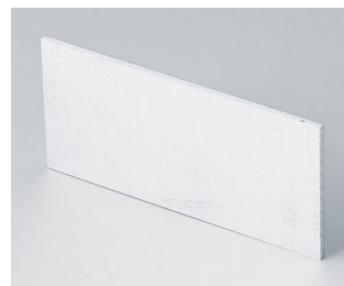
B6121111 Front panel Aluminium matt anodised 67.7x31.6x1.5mm
