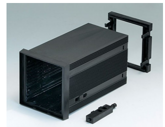
B6023061 DIN-MODULAR CASE TYPE A PPO (UL 94 V-0) black RAL 9005 72x72x124mm
