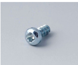
A0305031 Self-tapping screws 2.5 x 6 mm (PZ1)
