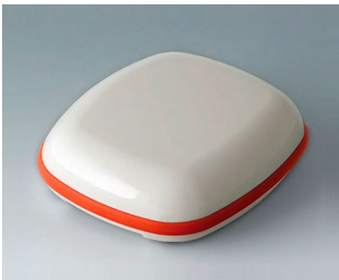
B1606107 BODY-CASE L, without recess ASA (UL 94 HB) traffic white RAL 9016 55x46x17mm IP 65
