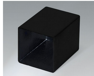
A8026358 POTTING BOXES, Vers. III PA 66 (UL 94 HB) black RAL 9005 26.4x26.4x35.2mm
