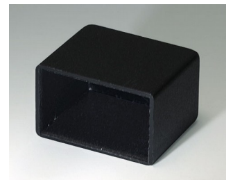
A8021178 POTTING BOXES, Vers. III PA 66 (UL 94 V-2) black RAL 9005 21.3x13.3x17.7mm
