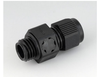
C2312919 Cable gland M12x1.5, pressure compensation PA black RAL 9005
