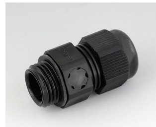
C2316919 Cable gland M16x1.5, pressure compensation PA black RAL 9005 IP 68
