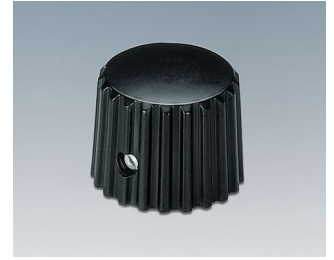
A1321160 TUNING KNOB, with lateral screw fixing ABS (UL 94 HB) black RAL 9005 20x16mm 6mm
