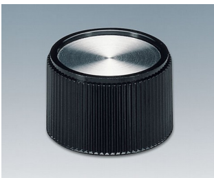
A1328160 TUNING KNOB, with lateral screw fixing PF (UL 94 V-0) black/alu 28x16mm 6mm
