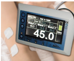
3D angle measurement of articulation systems on a gravity basis
